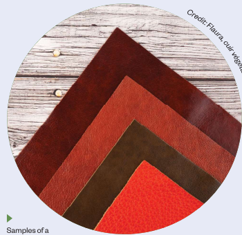
Samples of a sustainable alternative to leather made from apple waste.
