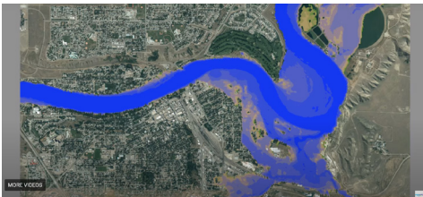
Calculated Flood Water Depth from Alberta Env. Flood Extents and 15 m Lidar
